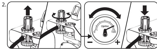
To adjust air pressure, pull up on the black Regulator Knob until you hear a "click." Turn the knob clockwise to increase air pressure ("+" sign), or counter-clockwise to decrease air pressure ("- " sign). When the desired pressure is reached, push down on the knob to lock it in place.
