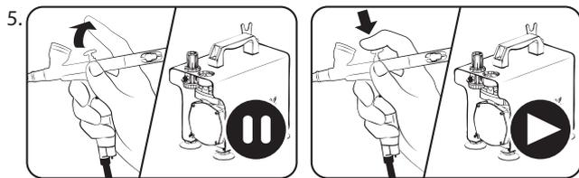
With a dual-action airbrush attached, but not in use, the Auto Stop Pressure Switch automatically stops the compressor when the pressure reaches 60 psi, and will automatically re-start the compressor when the airbrush trigger is pushed down and the pressure drops to 40 psi. Do not attempt to remove the Auto Stop Pressure Switch. In the rare instance that the switch malfunctions, do not allow the compressor to operate above 80 psi, and run the compressor continuously no more than 40 minutes.
